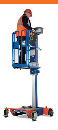
Only trained, authorised operators should use this platform. All operators must read and comply with the following Operating Instructions and Safety Guidelines before using the Pecolift Wind Rated (WR). This platform is designed for safe access to a maximum working height of 3.5m for 1 person + tools (150kg safe working load) and is for indoor or outdoor use.
