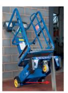
Ensure you use a safety prop which is 660 mm in length and place this under the corner of the chassis by either of the rear rubber pads to prevent the machine toppling back, this is indicated by the red arrow.
