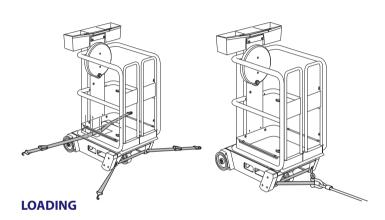
If loading with the aid of a winch up a ramp to the trailer, connect the winch cable to the castor/gate end of the chassis using the location holes provided. First run a strap through the holes, and then connect the winch cable to the strap.
