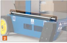
Emergency lowering tool located on chassis
